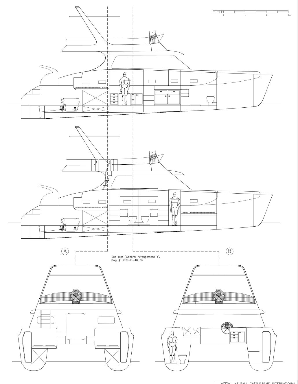
The aft cockpit is full width with direct access from the transom steps. The main berths are in twin aft cabins. Large capacity fuel tanks are arranged under these berths, giving a maximum range of 2000 nautical miles. This can be increased with extra tankage. The forward cabins are within the hulls. Saloon with galley and inside steering are on the bridge-deck.
